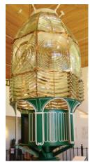
As we wait patiently for the arrival of our 4th Order Fresnel lens on loan from the Coast Guard, you can learn more about how a Fresnel lens works. A Fresnel lens consists of a series of "flash panels" attached together in a rough circle. Each flash panel consists of a central convex lens with prisms placed above and below this "bull's eye". The prisms bend (refract and reflect) rays of light and focus them into a specific direction, which makes the light much brighter.
