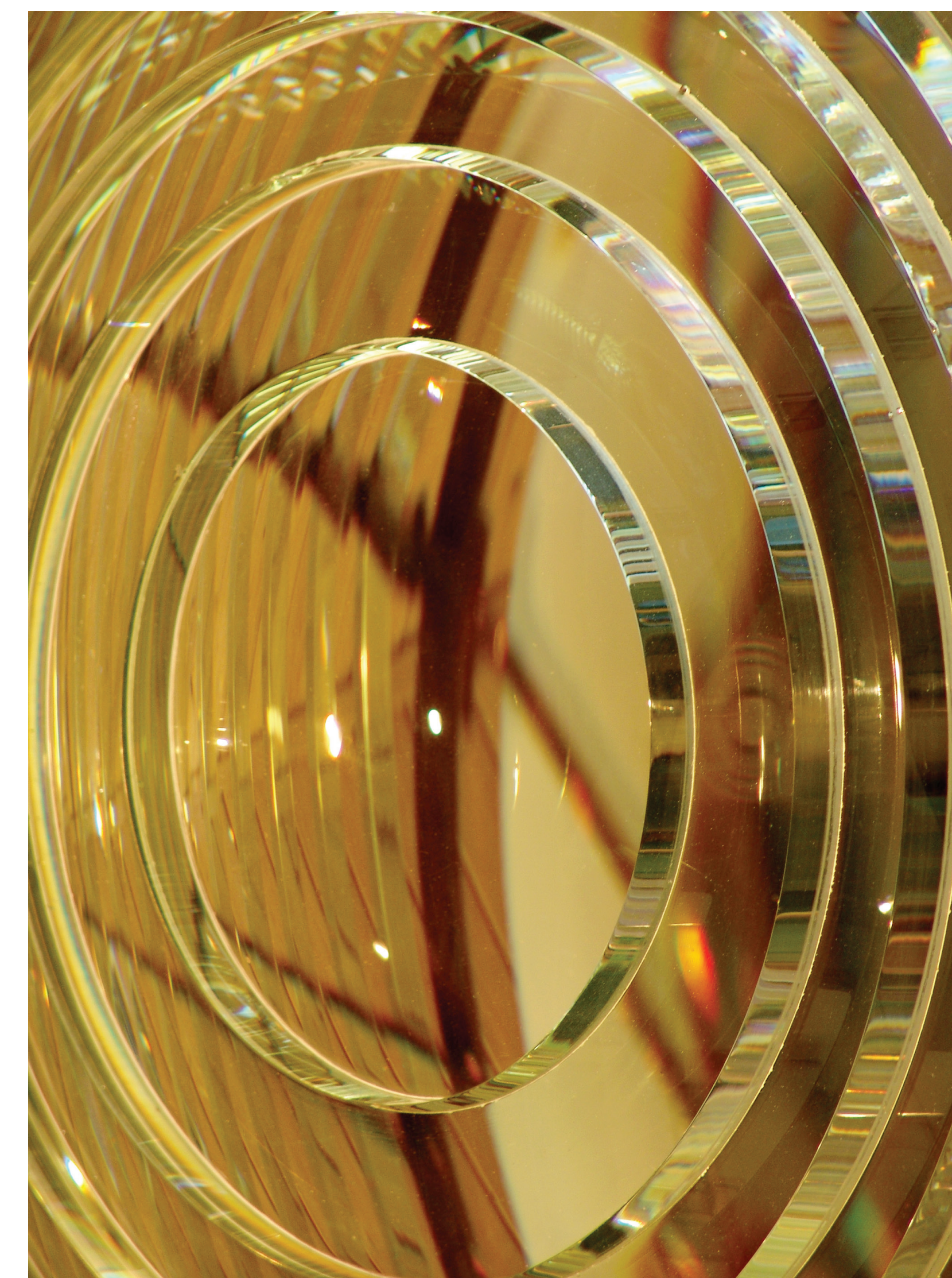
Bulls eye of the 1st Order Fresnel Lens
